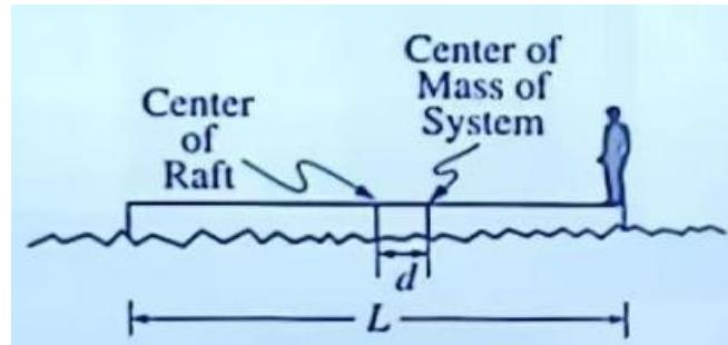
If friction between the raft and the water is negligible, how far does the raft move relative to the water?
